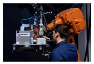
Fuel cell technology was considered a niche market for a long time. Due to the transition phase in energy generation and the search for alternative drives, the market demand might grow notably. For efficient mass production an increase of throughput in welding of metal bipolar plates, used to build the stacks in a fuel cell, is needed. High welding speeds require fast scan systems and high power
