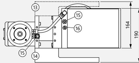
Objective  $f = 460$  mm and QBH fiber adapter
