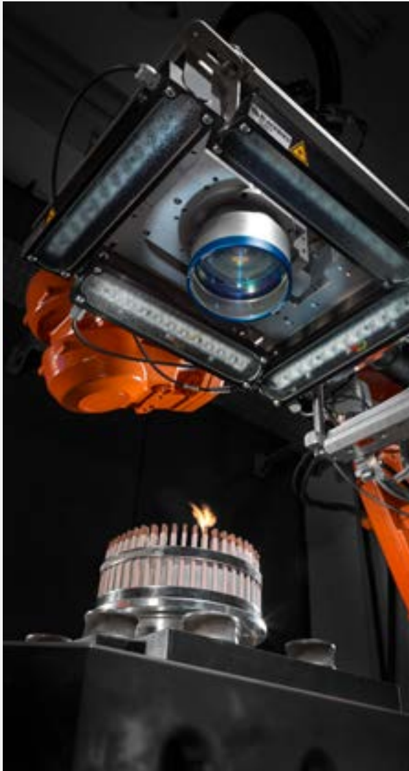
Hairpin welding during stator production – a common process in e-mobility
