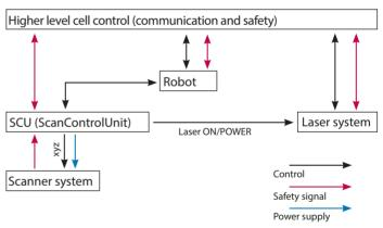
In a laser system, the SCU is integrated into the safety circuit of the overall system (interlock, emergency stop) to ensure safe system operation.
